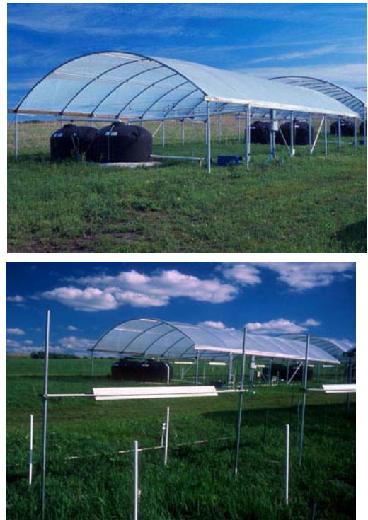
Figure 3. Top: View of one of the Rainfall Manipulation Plots (RaMPs) prior to installing IR lamps. Bottom: IR heating lamps in a reference plot in the foreground. See text for a more detailed description of the shelter design and operation.
